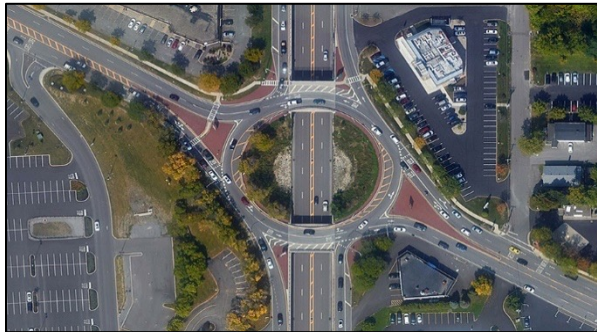
SPUI with Roundabout
